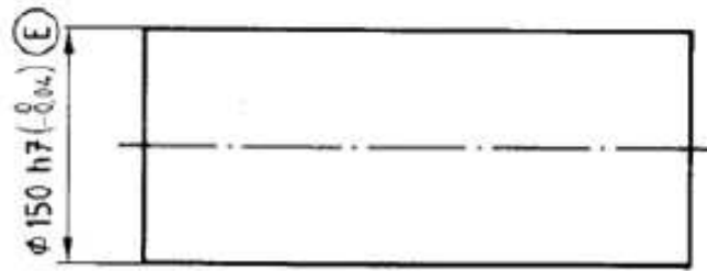
Figure A.16 – Envelope requirement drawing note
