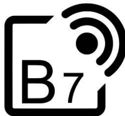
Figure 5: Symbol identifying products with RFID identification according to ISO 17367
